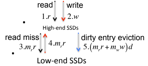
Fig. 2. A mixed SSD array with LRU caching policy (red line: writes in cache, blue line: writes in main storage)
