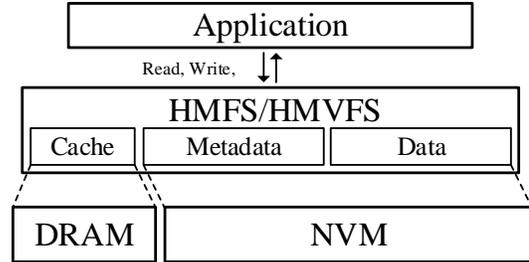
Figure 2. Architecture of HMFS/HMVFS
