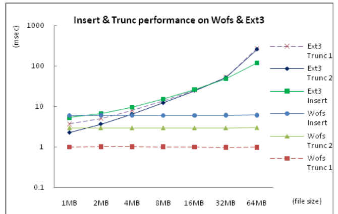
Figure 10. The time needed for doing 1 insertion and 1 truncation on Wofs with different file sizes ignoring the time needed for network communication, and the time needed for doing 1 insertion and 1 truncation on ext3 with different file sizes.
