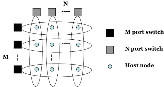
**Figure 1.** A 2 dimensional  $M \times N$  hybrid design composed of  $M$   $N$ -port switches and  $N$   $M$ -port switches. Each storage node is required to have 2 ports.
