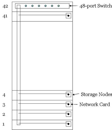
**Figure 3.** A 41-node one-dimensional hybrid cluster using a standard 42U rack.
