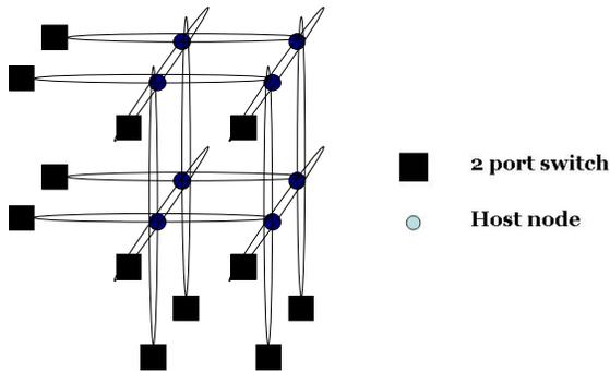
**Figure 2.** A  $2 \times 2 \times 2$  3D hybrid storage cluster.
