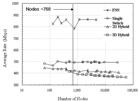
**Figure 6.** Average bandwidth vs. node count when the number of flows across the network equals the node count. The 2D and 3D Hybrid models are our designs.
