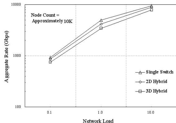
**Figure 7.** Aggregate bandwidth when the number of flows is  $1/10^{\text{th}}$  the node count, equal to node count and 10 times the node count when the node count is 10,000.
