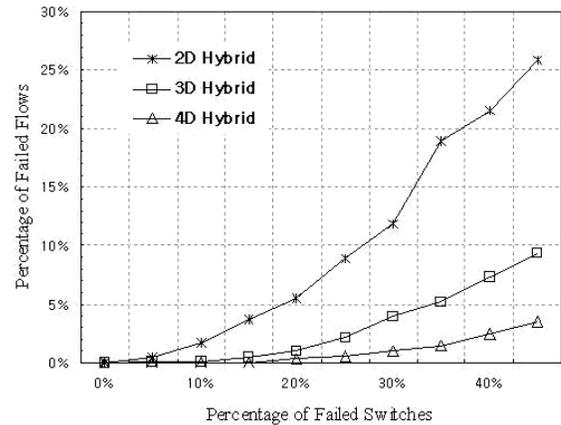
**Figure 9.** Percentage of failed flows for our proposed hybrid models. The node count used is 4096, with flow count being ten times the node count.
