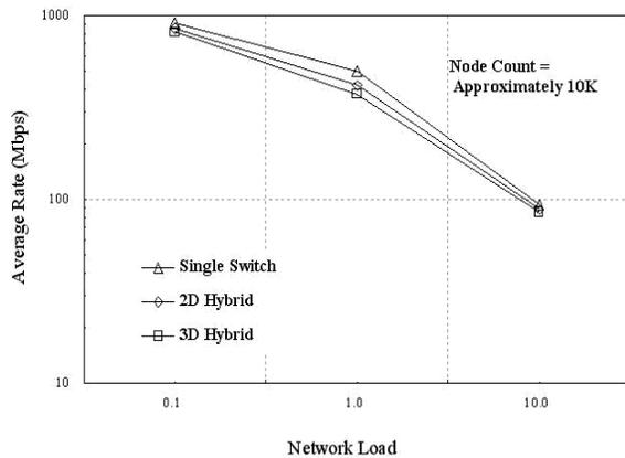
**Figure 8.** Same data as Figure 7, but plotting average bandwidth per flow when the number of flows is  $1/10^{\text{th}}$  the node count, equal to node count and 10 times the node count when the node count is 10,000.
