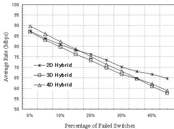
**Figure 10.** Average rate in the presence of switch failures.
