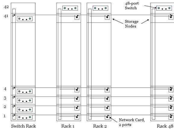
**Figure 4.** A two-dimensional hybrid model built using 49 standard 42U racks: the switch rack contains 41 switches with 48-ports each and racks 1 through 48 are copies of the racks in Figure 3 and contain 1 switch and 41 nodes each. The end result is a cluster of 41 x 48 storage nodes.
