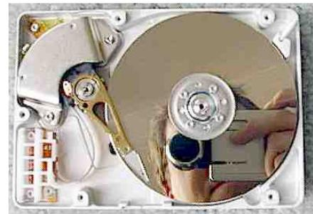
**Figure 1. Typical Multi platter Hard Disk Drive**
