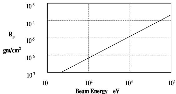
**Figure 7. Practical Range  $R_p$  vs. Beam Energy**
