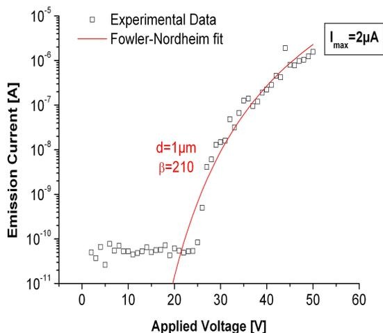
**Figure 5. CNT Emitter Current vs. Voltage**
