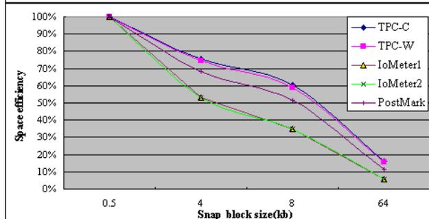
Fig. 9 Space efficiency as a function of snap\_block size
