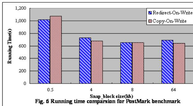
PostMark results are shown in Figure 6 in terms of total running time for 100,000 transactions on 50,000 files. For this benchmark, it seems that the two snapshot methods show similar performance across all block sizes considered with the difference less than a few percents. One observation that is consistent with all other benchmarks is that the performance of 512B snap\_block size is not as good as other block sizes. This observation suggests that using sector size to do snapshot is not an
