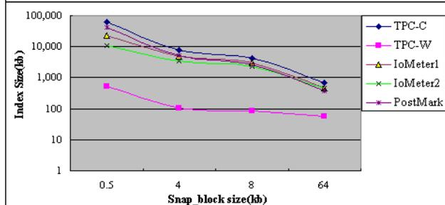
Fig. 8 Space required for index structure (in logarithmic scale)
