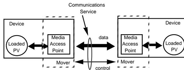
Figure 3. MSSRM Concept of Mover Architecture, "PV" is "Physical Volume"
