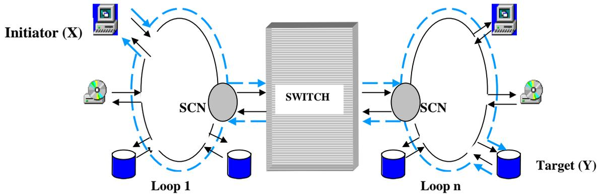
Figure 1: The simulation model for the circuit Switching based approach.
