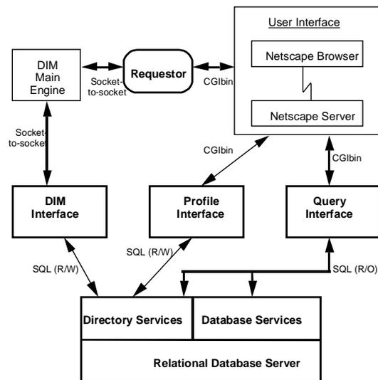
Figure 7. Anatomy of Database Subsystem
