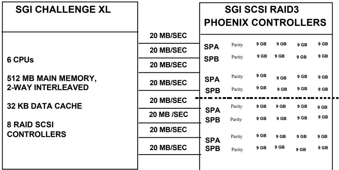
**Figure 7. Archive Hardware Configuration Under Test as of August, 1997**
