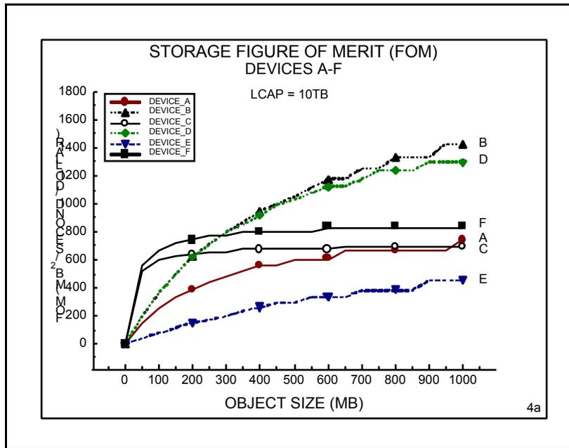
Figure 4a. Storage Figure of Merit in units of (MB<sup>2</sup>/second/\$). Devices A-F. Library capacity is 10.0 TB. Aggregate effective data rate is 20 MB/second. See text.
