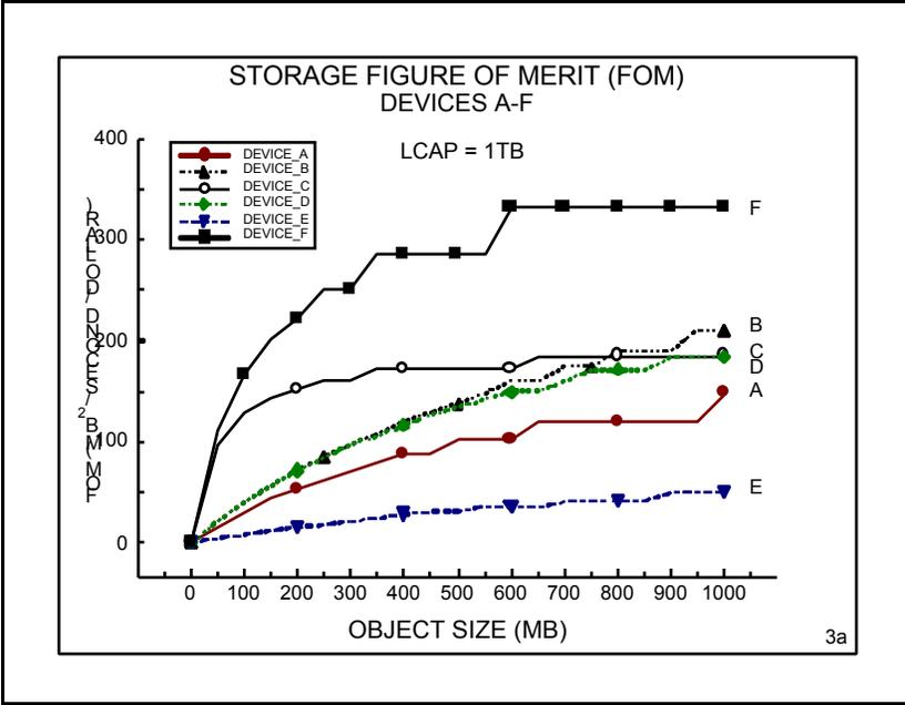
Figure 3a. Storage Figure of Merit in units of (MB<sup>2</sup>/second/\$). Devices A-F. Library capacity is 1.0 TB. Aggregate effective data rate is 20 MB/second. See text.
