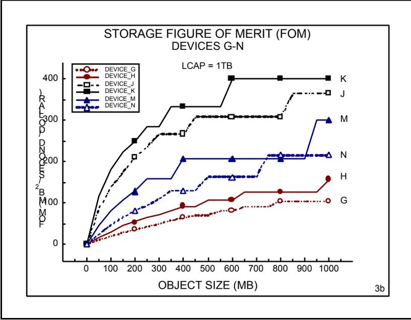
Figure 3b. Storage Figure of Merit in units of (MB<sup>2</sup>/second/\$). Devices G-N. Library capacity is 1.0 TB. Aggregate effective data rate is 20 MB/second. See text.
