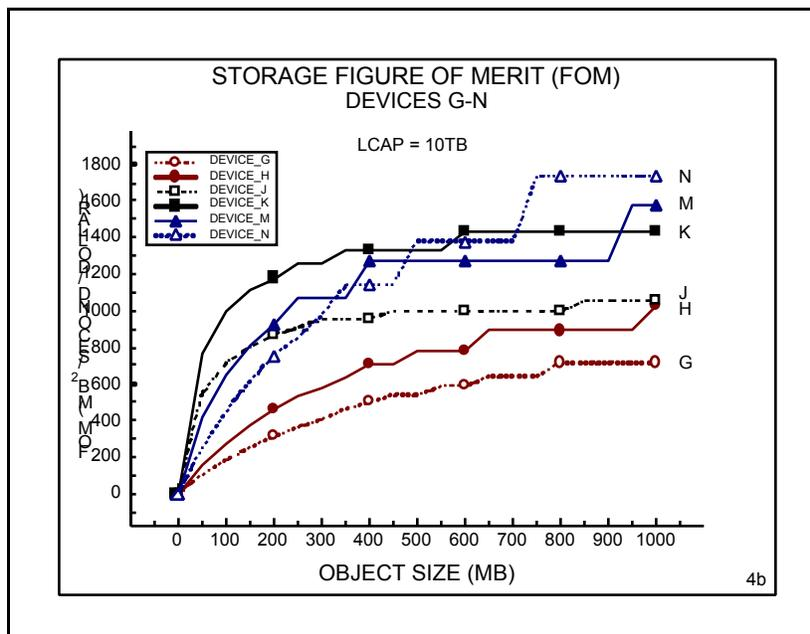
Figure 4b. Storage Figure of Merit in units of (MB<sup>2</sup>/second/\$). Devices G-N. Library capacity is 10.0 TB. Aggregate effective data rate is 20 MB/second. See text.
